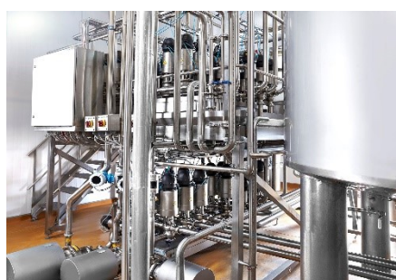
Automated milk pasteurisation process – a potential risk source
